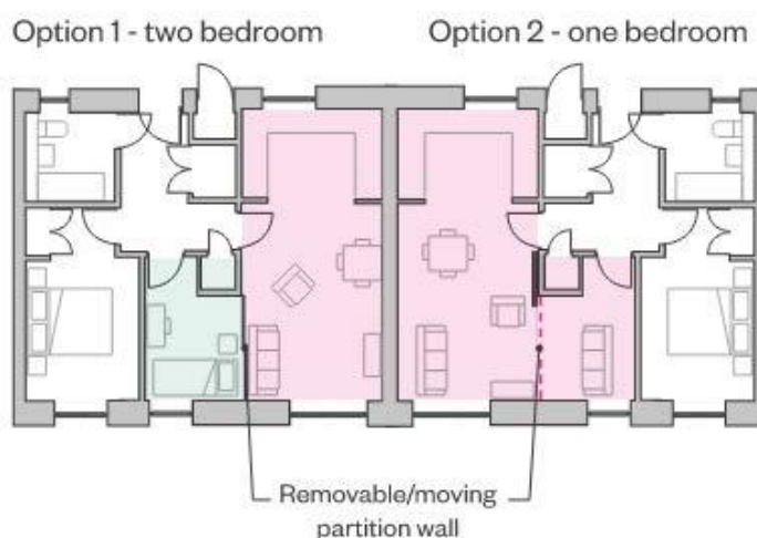
Figure 12: Design for adaptation using a flexible floor plan e.g., one bed flat can be converted to a two bed flat or a one bed flat with space for home working.
